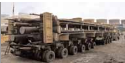
Below: a module is delivered by trailer before transfer onto the 'strongback'.
