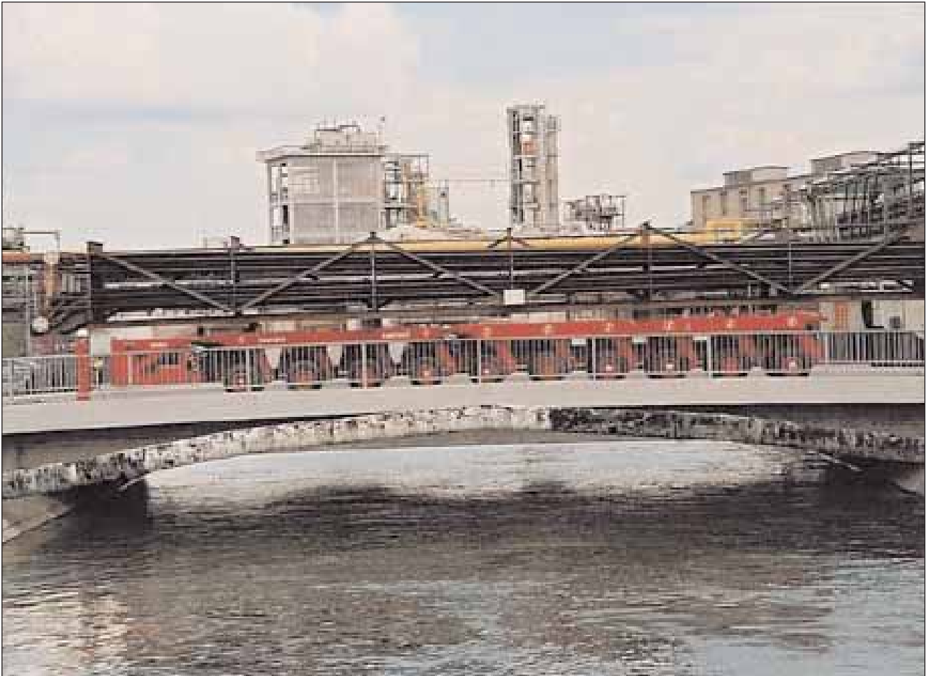
Above: Boiler Module on a 10 tonne SPMT (self propelled modular transporter)
