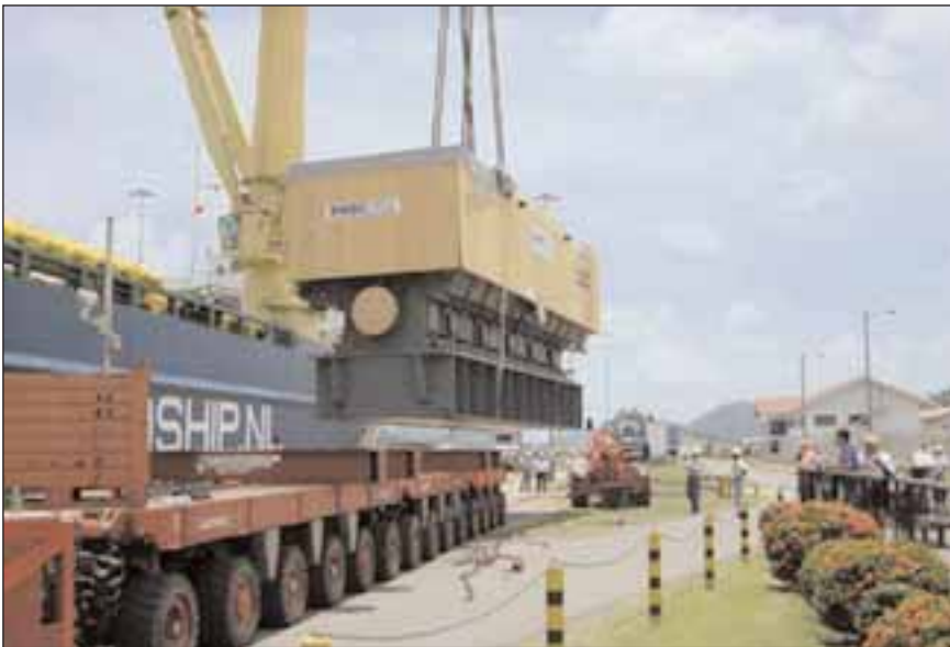
Above: Loading of the diesel engine onto the trailer.
