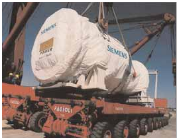
Above and below: Fagioli's ship 'Storman Asia' lifting one of the heavy lift components onto a SPMT using one of the Derrick cranes. The Derrick cranes have a capacity of 400 tonnes each.
