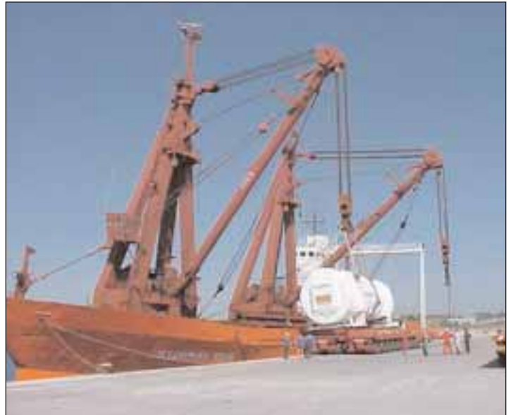
Above and below: Fagioli's ship 'Storman Asia' lifting one of the heavy lift components onto a SPMT using one of the Derrick cranes. The Derrick cranes have a capacity of 400 tonnes each.
